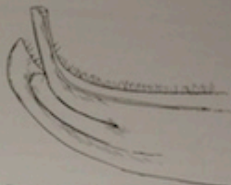
Figure 138. Bow of the Danish National Museum's Ib.160. Note the whiskers sewn into the longitudinal seams.
